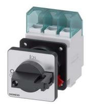
SENTRON, Switch disconnector 3LD, main switch, 3-pole, lu: 25 A, Operating power / at AC-23 A at 400 V: 9.5 kW, front-mounted, knob-operated mechanism, black, central mounting 22.5 mm of the handle
