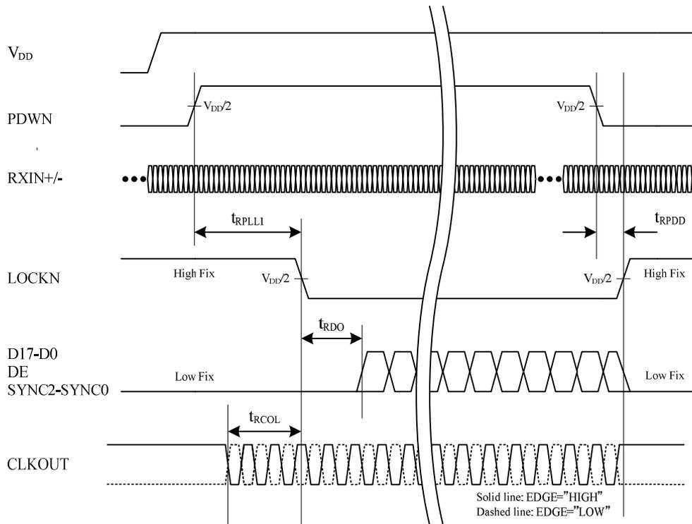
Fig. 9 Receiver Start-up and Power-down Sequence (THCV214)
