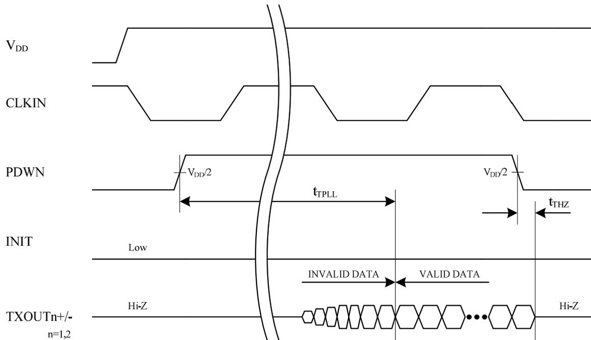
Fig. 7 Transmitter Start-up and Power-down Sequence (THCV213)
