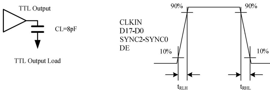
Fig. 4 CMOS/TTL Outputs Load and Transition Time (THCV214)
